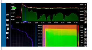
VeriCure software is tailored for CIPP installation professionals. Real-time data viewing allows you to monitor and control the cure for maximum quality and efficiency. VeriCure software also ensures that each zone has met and maintained the proper cure temperature while also monitoring cool down. The final data is summarized in a gradient chart to show temperature change over time.
